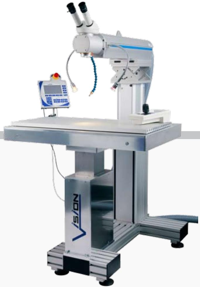
The Workstation T-Base V2 expands your FLEXX, turning it into a compact, open welding station with a digitally-controlled three-axis work table and a separate height-adjustable laser head.
